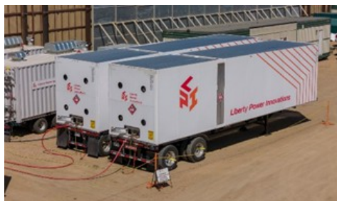
Figure 3: CNG Delivery Asset (Virtual Pipeline Solution via Trailer-Mounted Units)
