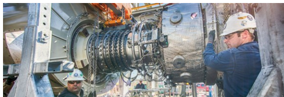
Figure 10: Solar Gas Turbine Overhaul
